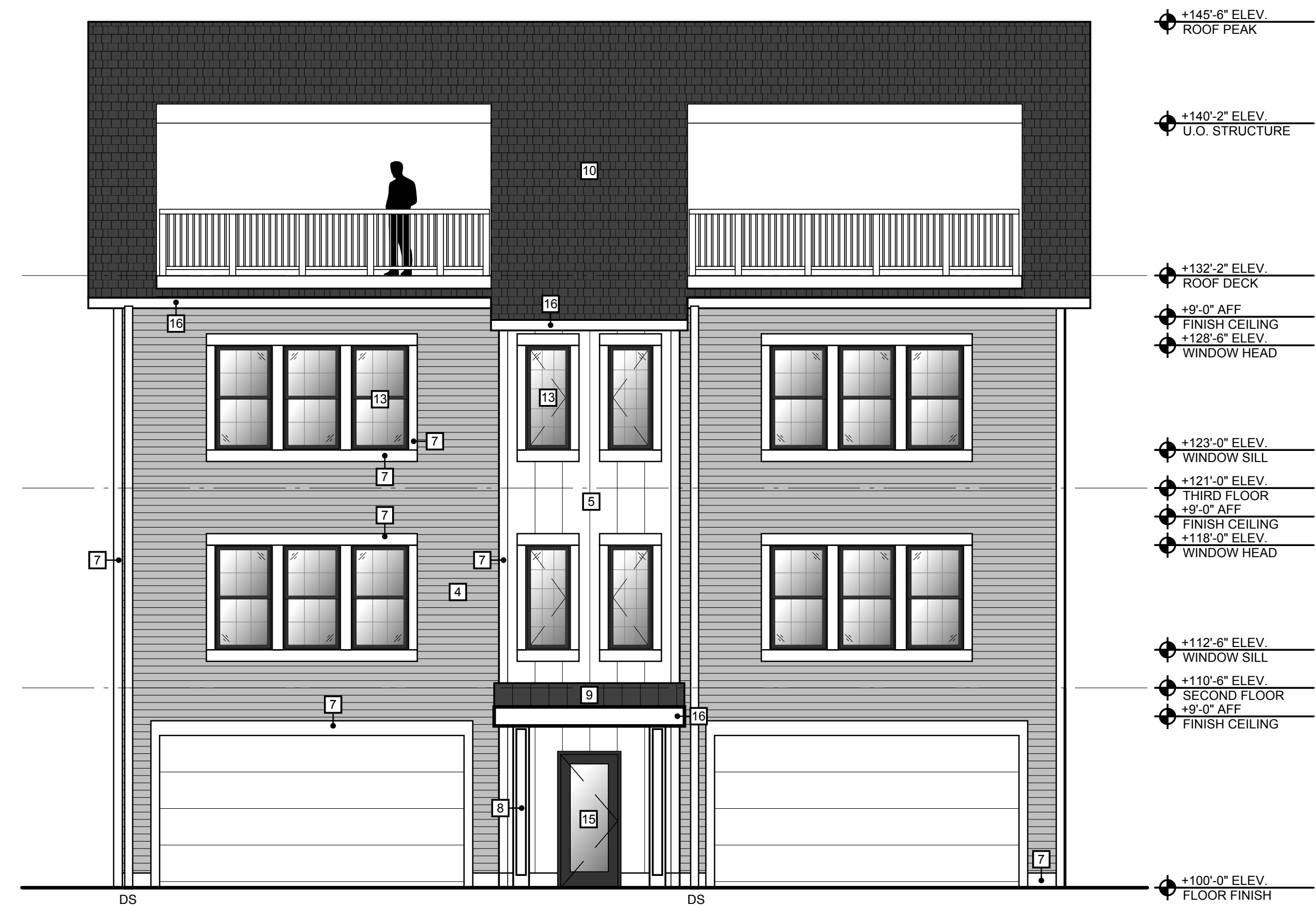
1. East Exterior Elevation
