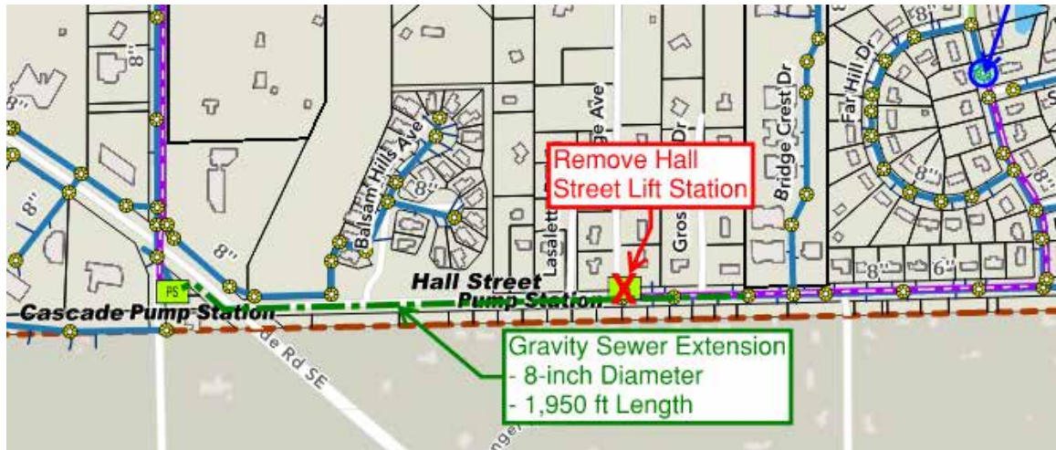
Figure 2 –Alternative B Gravity Sewer Extension Routing
