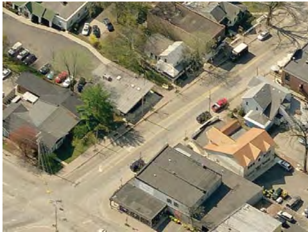
Figure IV-2. Left-hand turn lanes in Ada Village are considerably longer than one finds in downtowns with more traffic, resulting in the loss of important curb parking.
