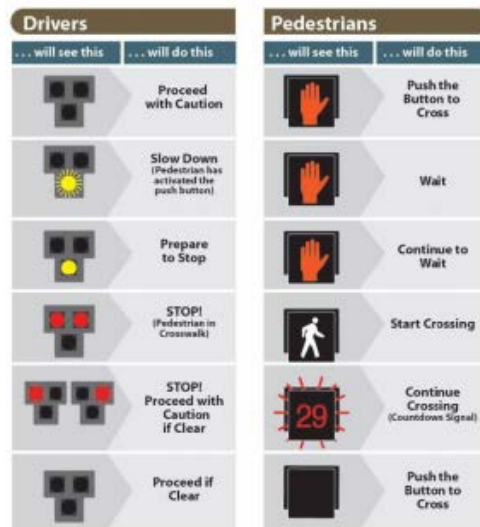
Pedestrian hybrid beacon phases Source: Michele Weisbart
