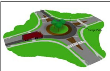
The center of a roundabout has an island, which is surrounded by curb that is mountable for larger vehicles.
